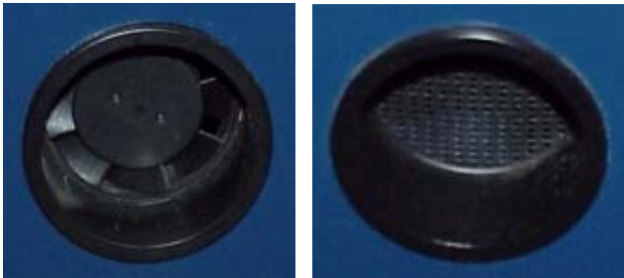
Left: Fan mounted on the right side of the box. Right: Vent mounted on the left side of the box.
